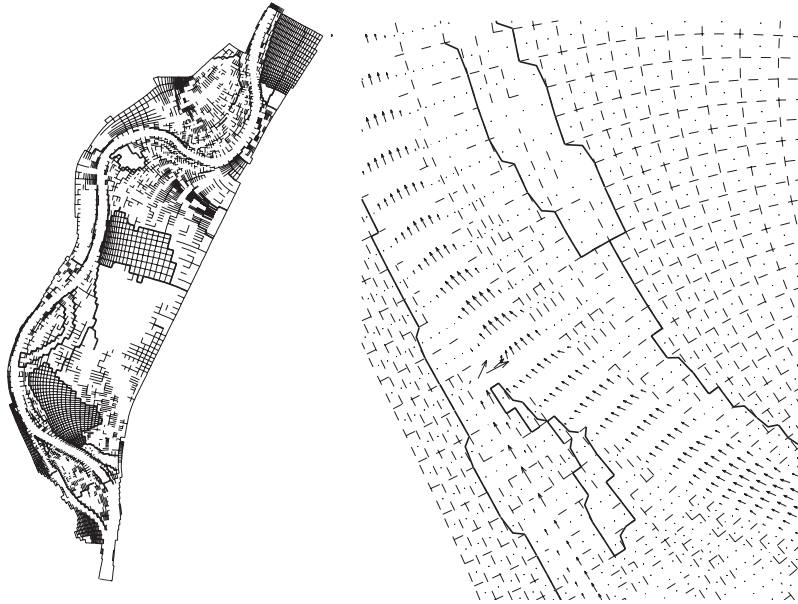
Figure 1. Illustration of screen-based wetting and drying methods for a part of the Meuse river in case of a flood wave due to heavy rainfall. Thick lines: weirs, model elements used to represent local strong bottom variations. Dashed lines: temporary screens placed to avoid flow at dry grid points.
